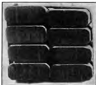
FIG. 84.—Copper imbedded in the surface of the brushes caused by sandpapering the commutator with the brushes down.
